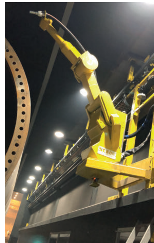
The side wall guided "ReCo-Blaster" in use
