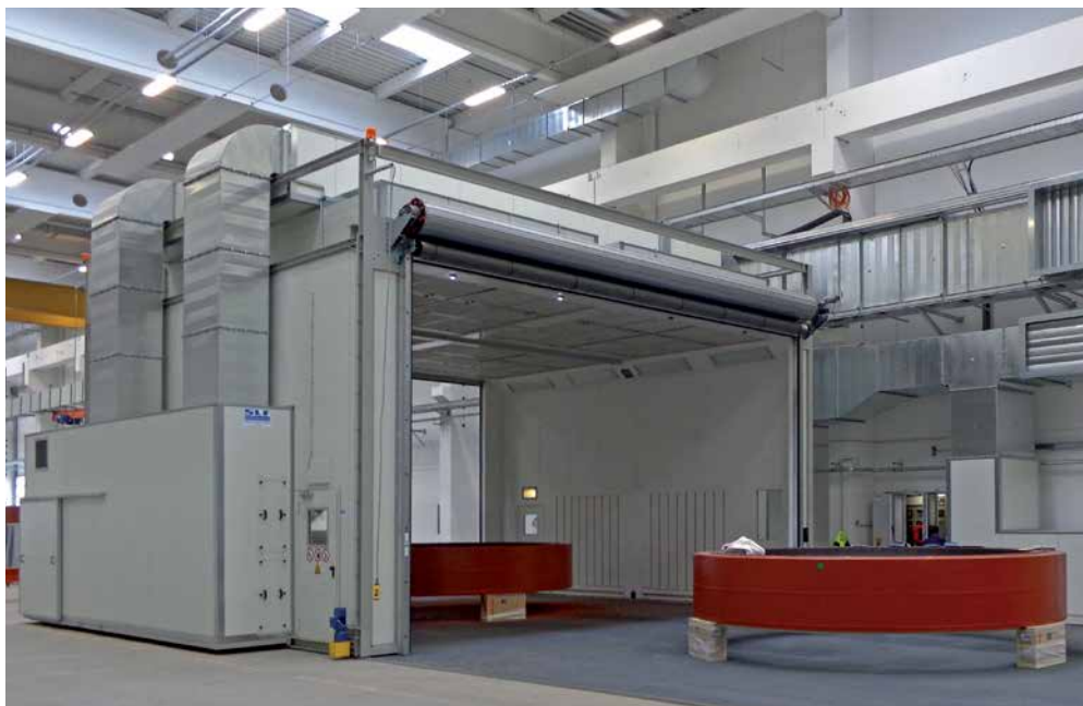
After the coating process the work pieces remain in the same place and the booth moves to a new working position.
