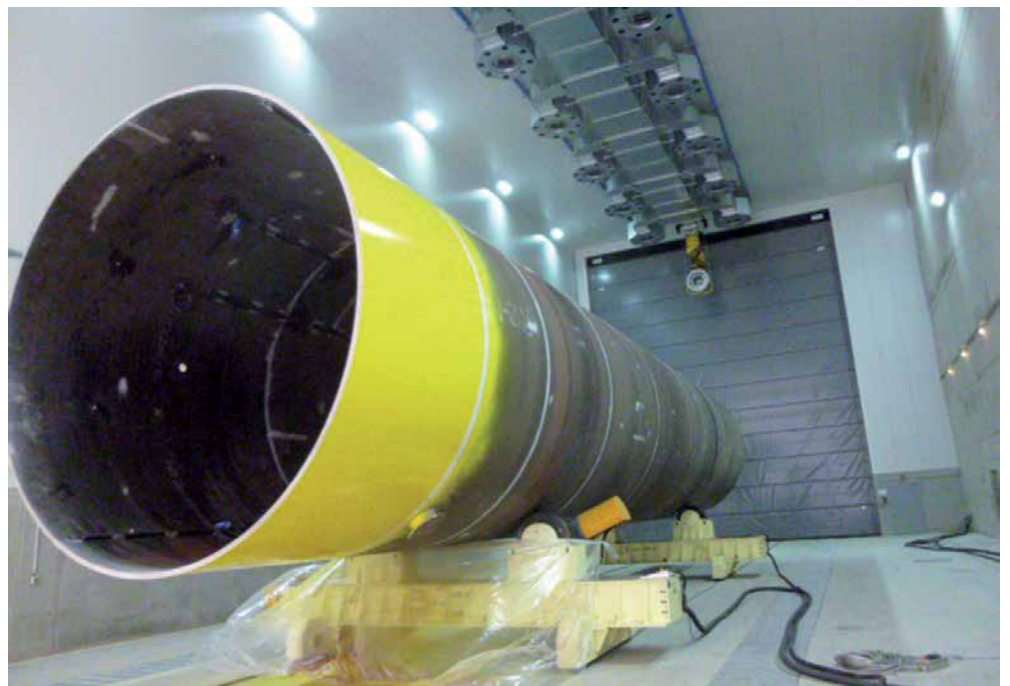
A monopile designated for an offshore wind power plant is painted in a booth with long-range nozzles.
