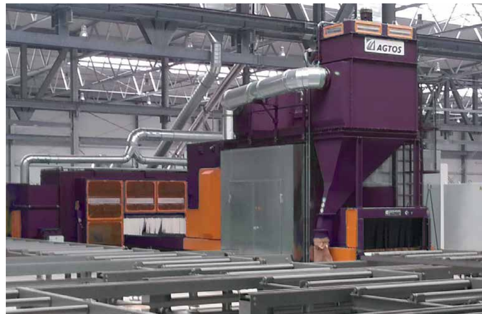
AGTOS roller conveyor blast machine with downstream paint spraying system and dryer.
