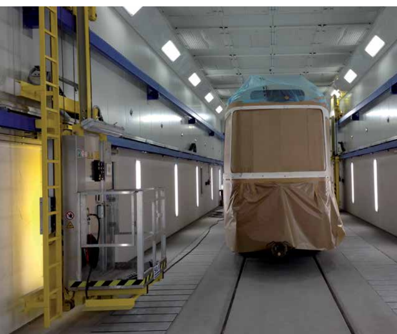
Tramcar in a combined paint spraying and drying booth before paint spraying.
