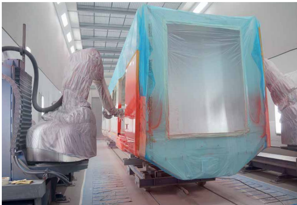
For the first time in Europe rail vehicles are painted with the help of paint spraying robots.
