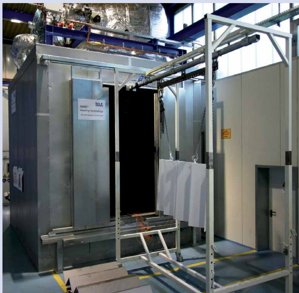
View of the DARC ® -type demonstration furnace developed and operated by us.
