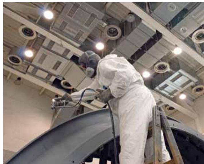
Perfect paint spraying of large components with an open-space paint spraying system.
