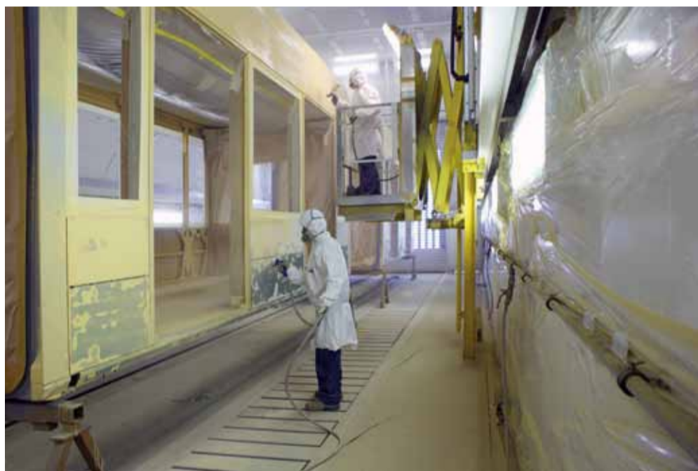
Optimum paint spraying using SLF lifting platforms.
