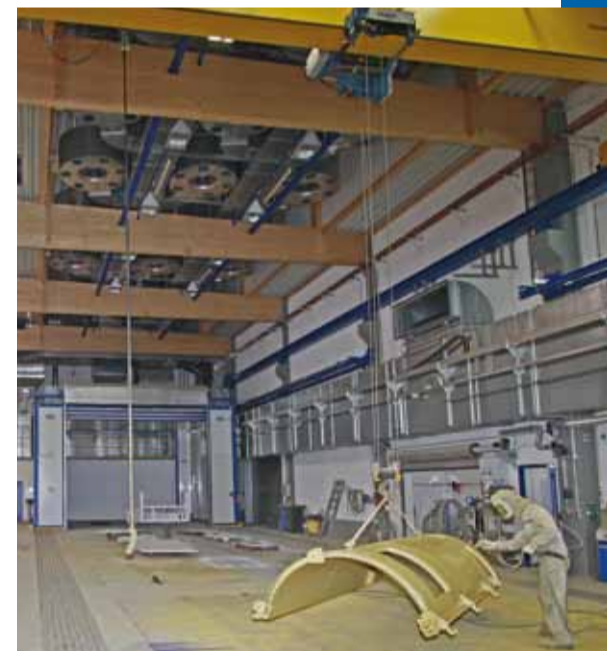
Open-space paint spraying area. In the background: Movable telescopic dryer in parked position.
