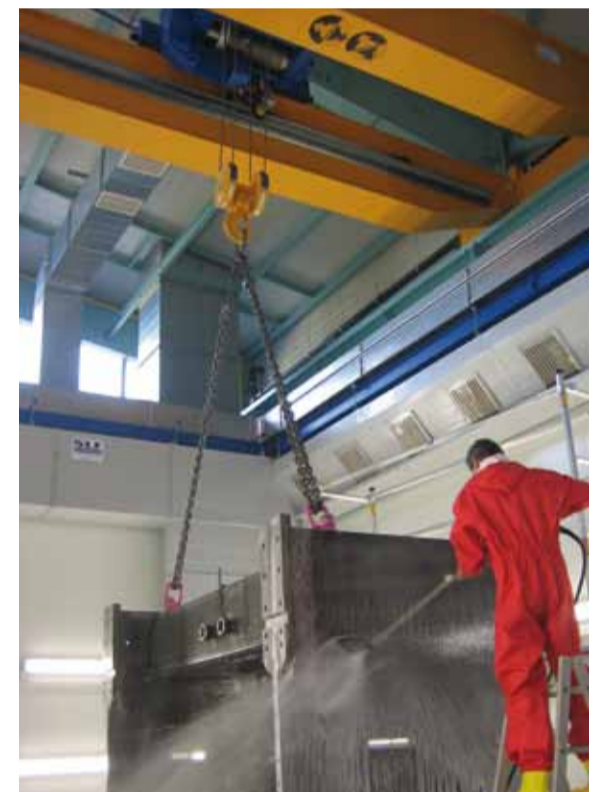
High-pressure cleaning cabin with ceiling opening for hall crane.
