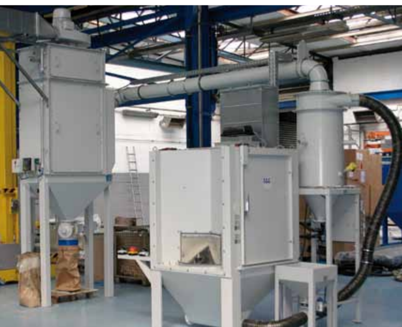
Automatic indexing table unit with direct suction system for the air blasting of synchroniser rings.
