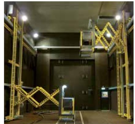
Scissor-type lifting platform in a blast booth
