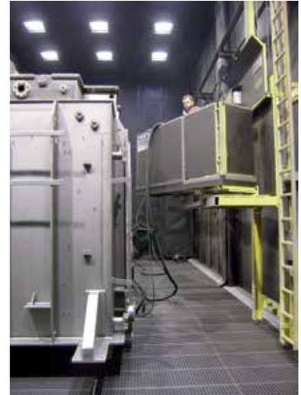
Swivelling lifting platform in a blast booth
