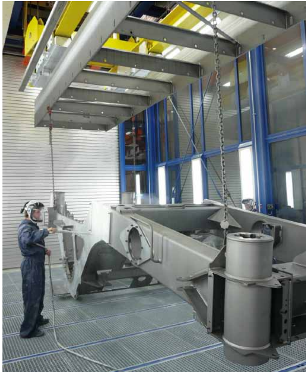
Powder coating of large components (Wirtgen GmbH)
