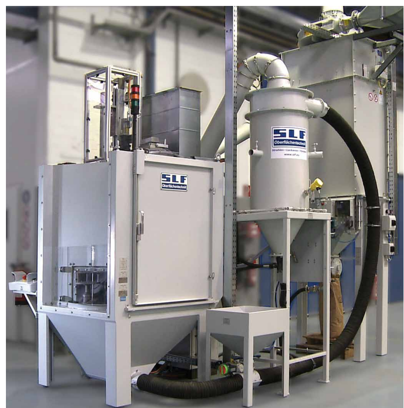
Automatic indexing table unit with direct suction system
