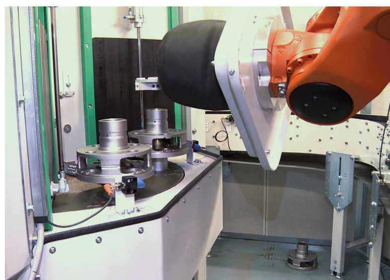
Pressure blast indexing table unit with automatic loading and unloading
