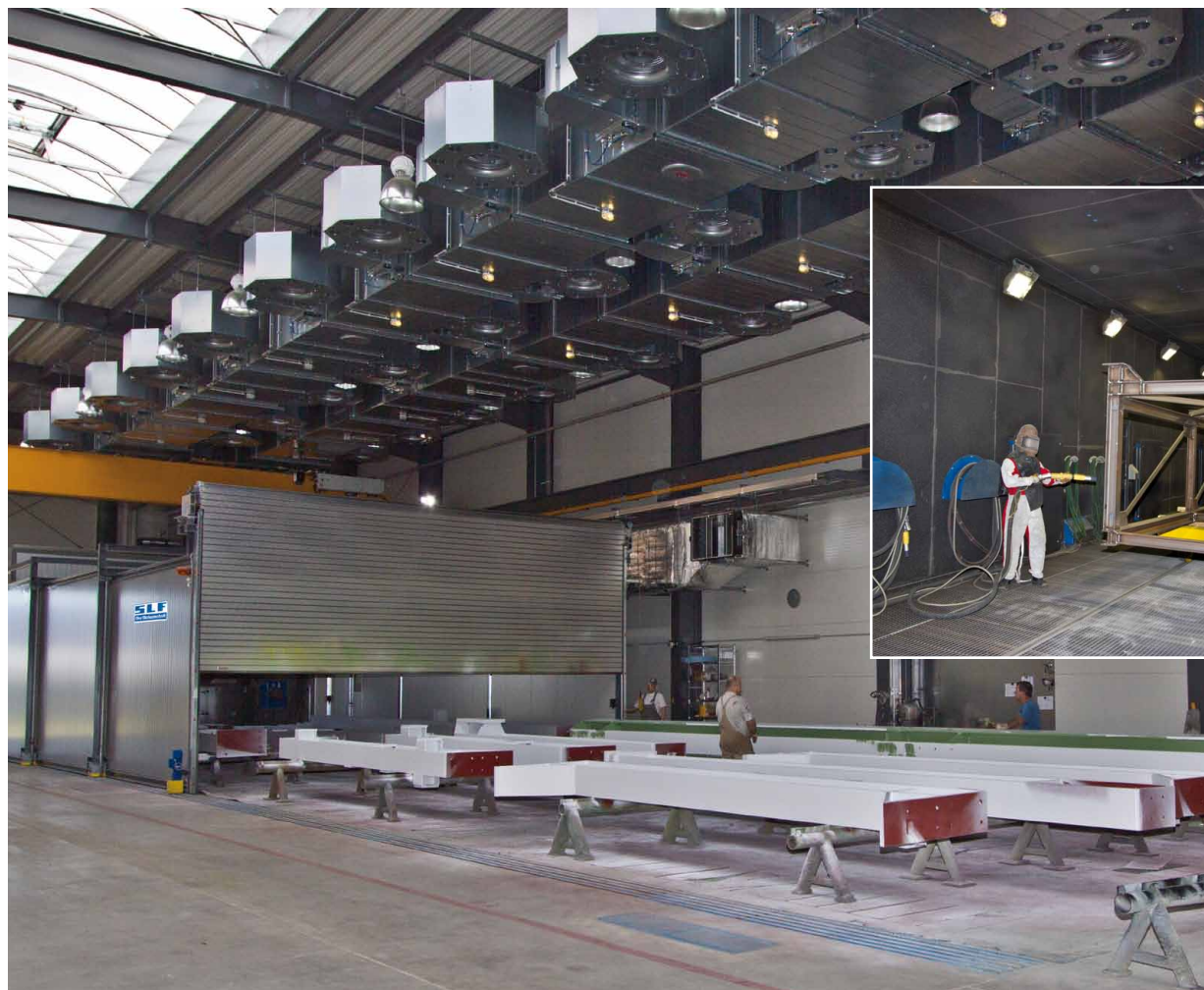
The most effective usage of open-space paint spraying systems: combination with a moveable telescopic dryer
