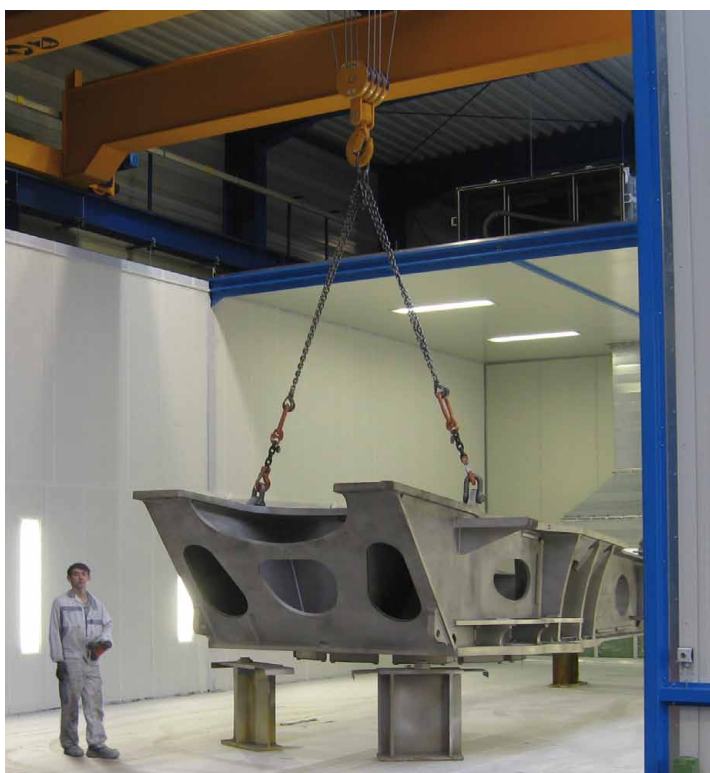
Loading of the twin cabin by using the bridge crane
