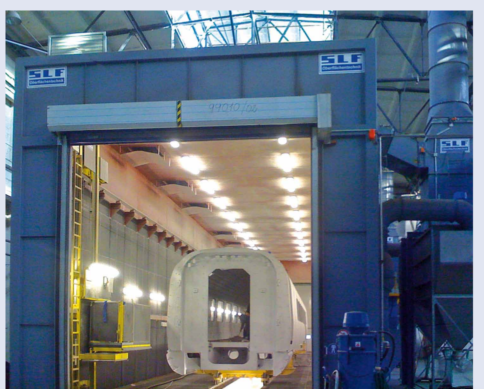
Blastroom for rail vehicles
