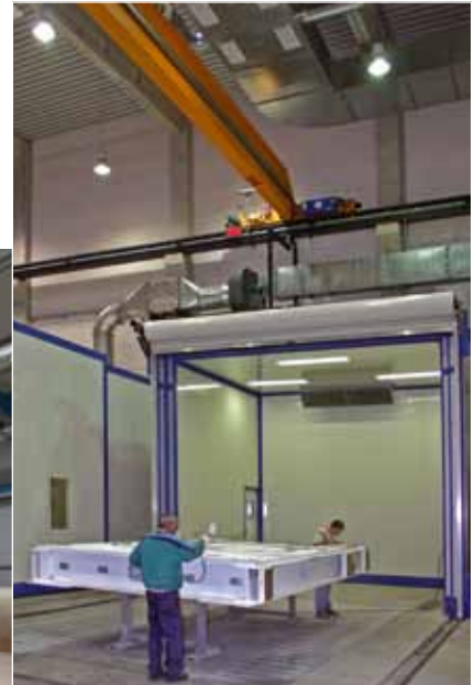
Open-space painting system with telescopic dryer.
