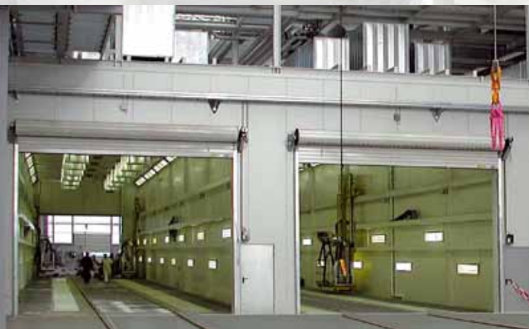
Combined painting and drying cabin with sectional ventilation by means of long-range nozzles for rotor blades.
