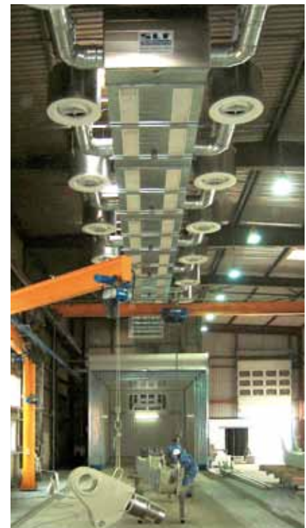
Open-space painting system with long-range nozzles and telescopic dryer.
