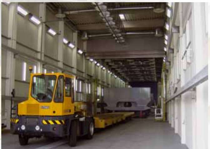
High-pressure cleaning room and combined painting and drying cabin with sectional ventilation system for large components.
