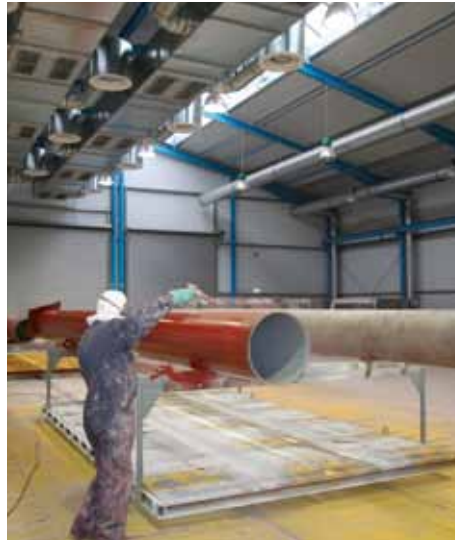
Open-space painting system for the multi-functional production.
