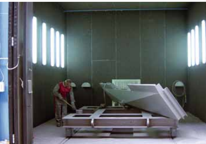
Blastroom for large components.
