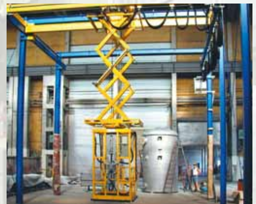
3-Axes telescopic platform for processing large components.
