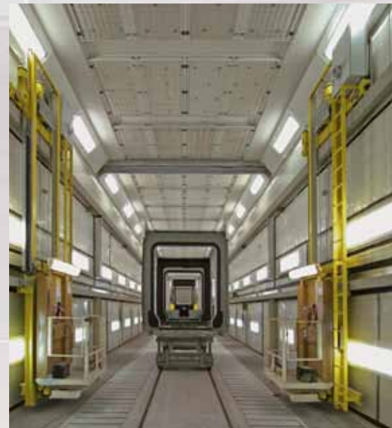
Combined painting and drying cabin with sectional ventilation system for passenger coaches.
