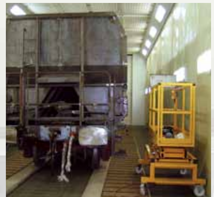
Combined painting and drying cabin for railway waggons.
