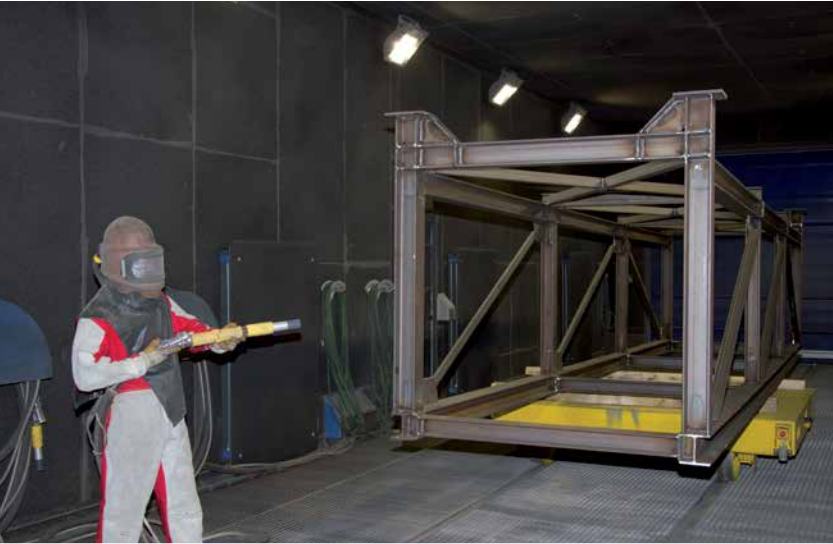
Depending on the task different blast media can be used in our blastroom.
