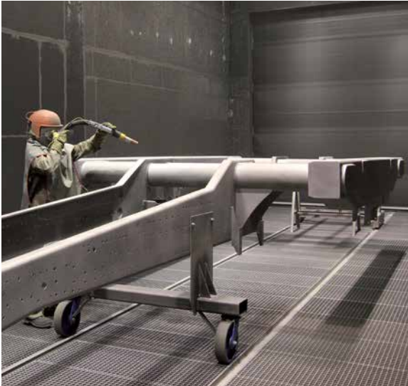
Blastroom with full-floor media reclaim system and ceiling crane for components of utility vehicles
