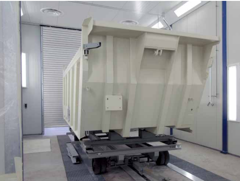
Work piece transport device connected to the floor-mounted chain conveyor in a paint spraying booth
