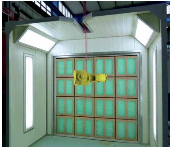
Open face spray booth with cardboard filters and crane slot for handling by a hall crane
