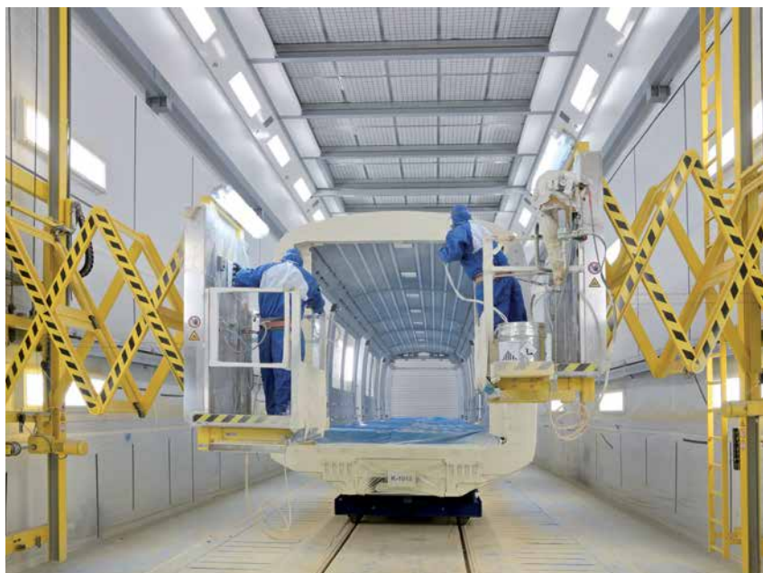
Combined paint spraying and drying booth for rail vehicles
