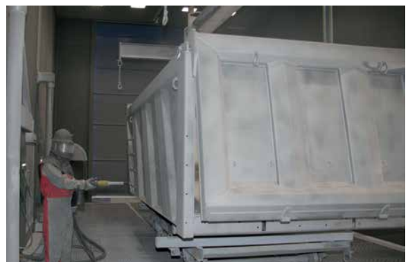
Blastroom with chain hoist
