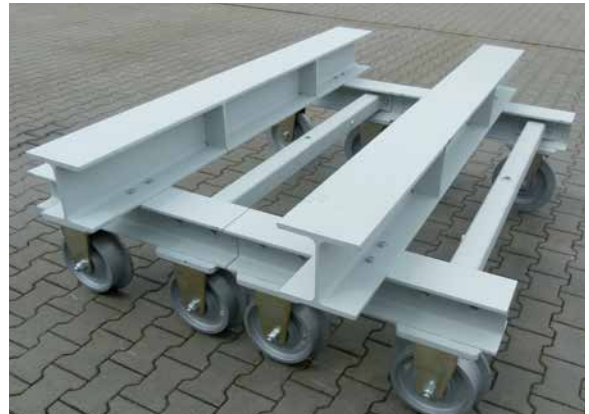
Two-part rail-bound trolley for manual work piece transport
