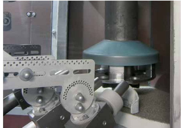
Blasting station for a shot peening machine
