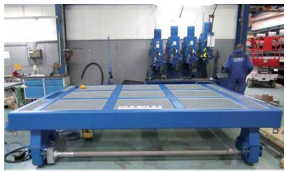
Electrically driven rail-bound trolley with lifting table
