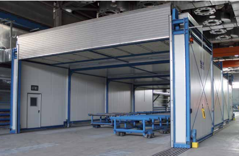
Movable and telescopic dryer with open-space paint spraying system
