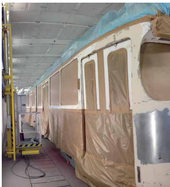
Combined paint spraying and drying booth for tramways and buses
