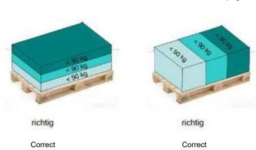
Non-slip layers of paper or cardboard must be placed between the pallet and the articles and between the individual horizontal layers of articles. Cardboard or a comparable (non-slip) material should also be used to separate vertical positioning blocks from one another.
