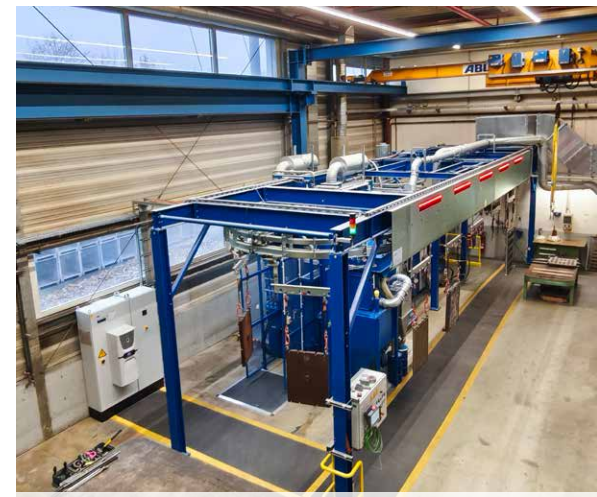
Continuous blasting system at the Boge plant in Damme
