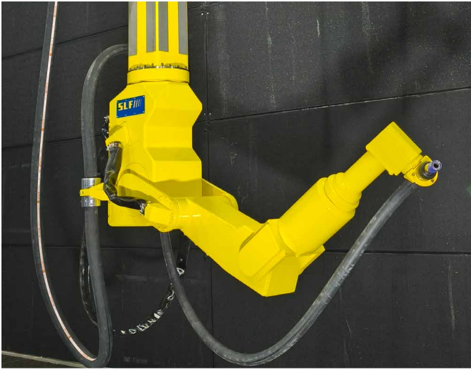
ReCo-Blaster® media blast robot in the blastroom at MEKON in Rastdorf
