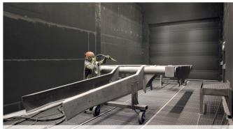
Blast cleaning of truck frame constructions with maximum precision in an **SLF** blastroom
