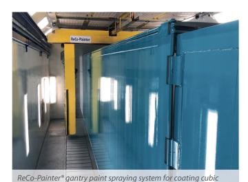
We have specially developed the ReCo-Painter®, an automated gantry paint spraying system for coating large, cubic components such as box bodies for trailers and containers with small undercuts, which enables automatic, efficient and reproducible coating with high spray precision. During system design, we focus on energy-efficient and technology easy-to-maintain that allows the system to be optimally integrated into your material flow.
