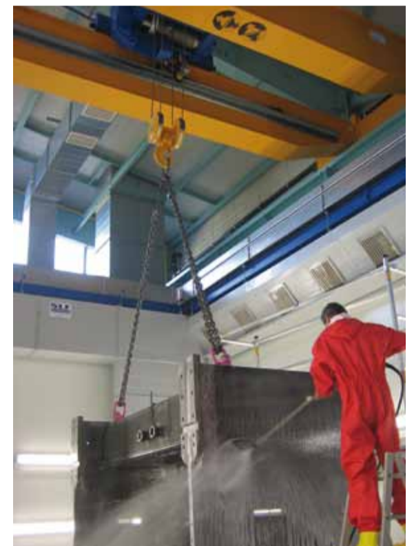
High-pressure cleaning cabin with ceiling opening for hall crane.
