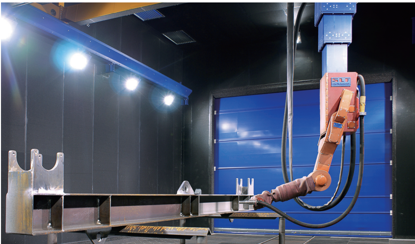
The ReCo-Blaster® - automatic blasting of large workpieces with high efficiency
