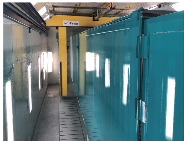
Efficient, automatic surface coating of cubical workpieces such as box bodies for trailers or containers with the ReCo-Painter®
