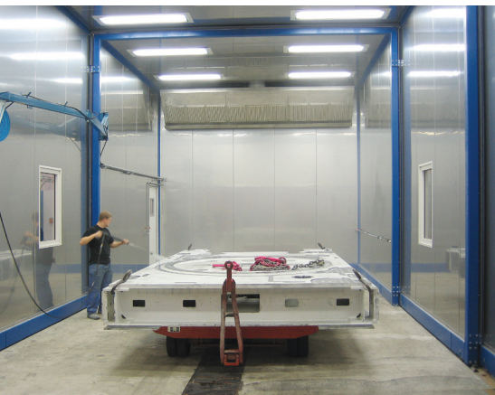
Telescopic cleaning cabin, length 12,5 m
