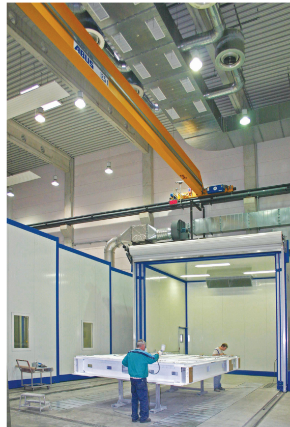
Open-space paint spraying system with long-range nozzles and telescopic cabin in parking position
