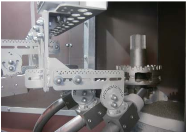
Five blasting nozzles blast the work pieces in exact compliance with several blasting process parameters
