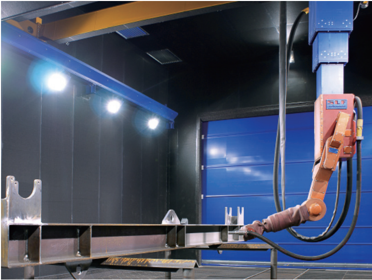
The "ReCo-Blaster" ® , a development of SLF blasts large work pieces, in particular serial and small serial parts, in a very time-efficient manner
